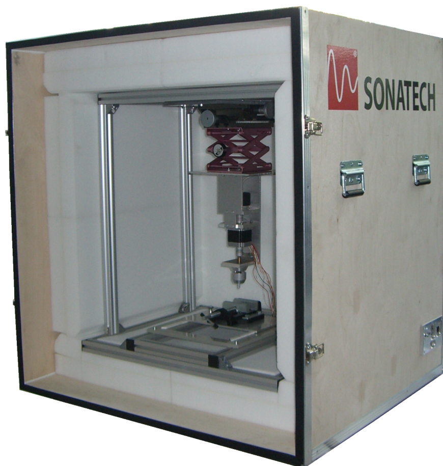
Figure 4.1: Final version of the actuation robot in its anechoic test box
