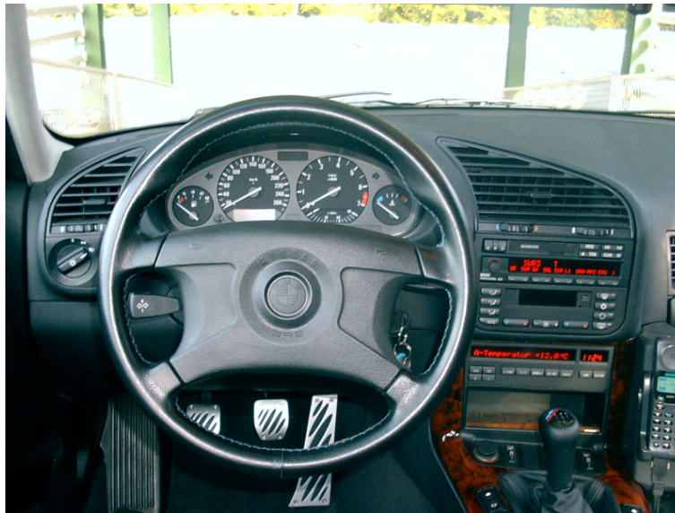
Figure 1.2: Dashboard of a BMW E36. Three displays on the center console, a mobile phone and over 30 control elements are needed to access each function - even without satellite navigation
