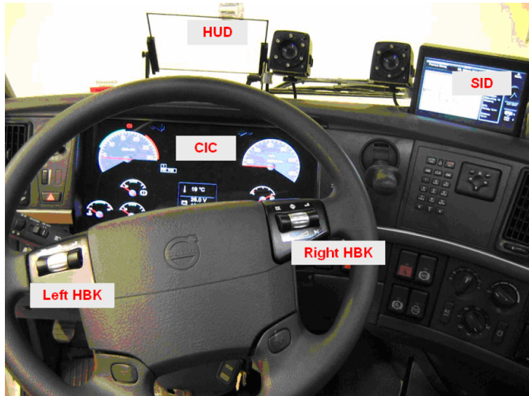
Figure 3.2: Prototype of an AIDE interface in a Volvo truck demonstration vehicle [27].
