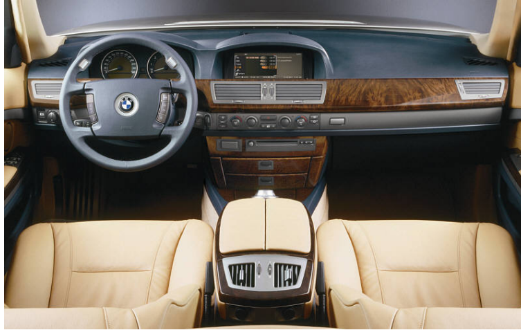
Figure 1.3: Dashboard of a BMW E65. One raised display close to the driver's line of sight as well as one large control element.
